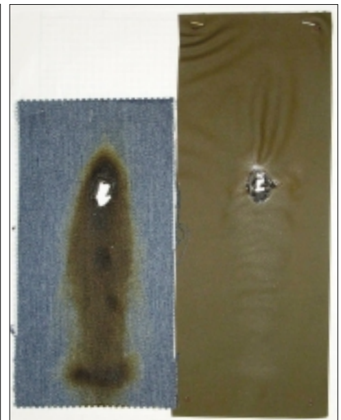
Fig 3. PVC film and specimen of a fabric made of Viscose FR, wool, and cotton (315 g/m 2 ). Tested with 208 g of aluminium
