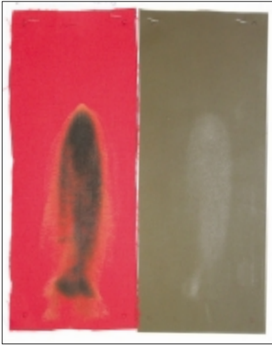
Fig 5. PVC film and specimen of a fabric made of Viscose FR and wool (300 g/m 2 ). Tested with 207g of aluminium
