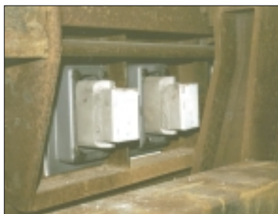
Collars for collector bars cast by Malmsteypa for Alcan
