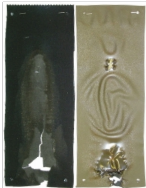
Fig 2. PVC film and specimen of Pyrowatex treated cotton (290 g/m 2 ). Tested with 213g of aluminium
